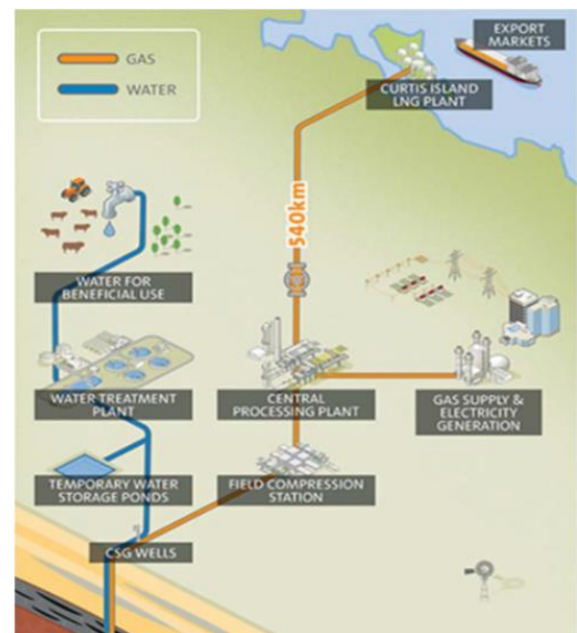
Figure 1: Schematic of the water and gas cycle for QGC operations
