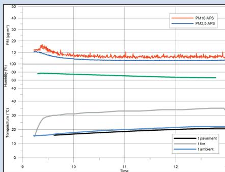
Figure 2. Particle concentration measured by APS, temperatures and relative humidity during the test of the silica-based summer tire.
