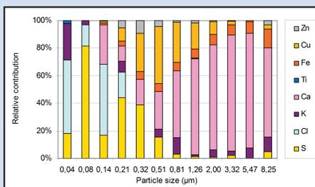
Figure 5b. PIXE analysis of airborne TWP with Si removed (Michelin Pilot Primacy shown)
