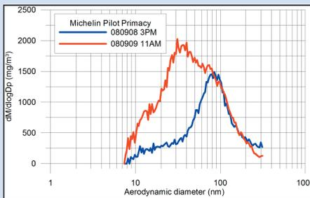
Figure 4. Selected particle mass size distributions from stable periods (SMPS)
