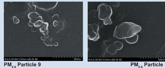
Figure 6. FE-SEM photographs of ultrafine airborne particles collected at VTI
